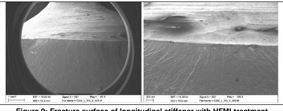
Figure 9: Fracture surface of longitudinal stiffener with HFMI-treatment
