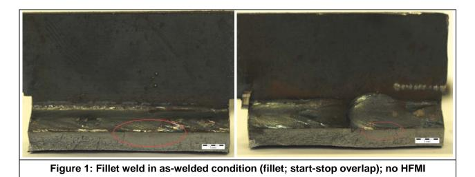
By use of the start-stop-overlapping seams as additional fatigue test lot it is possible to study the effectiveness of HFMI-treatment quality on fillet welds which may also possess local weld process based heterogeneities. Such start-stop ends occur in commercial workmanship environment tasks regularly.
