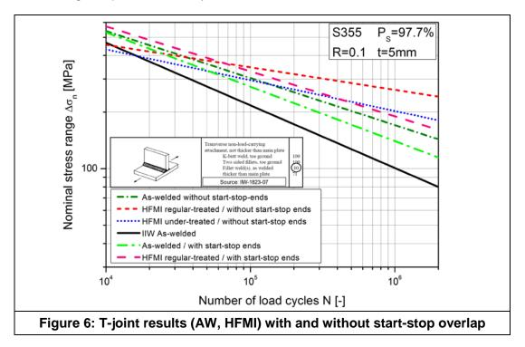
Whereas the geometric heterogeneity of the start-stop end region has a significant effect on finite fatigue strength, a regular-treated HFMI process is capable to enhance the both S/N-curves. Proper HFMI-treatment leads to a unification of, comparably small, weld process manufacturing effects into a single design curve.
